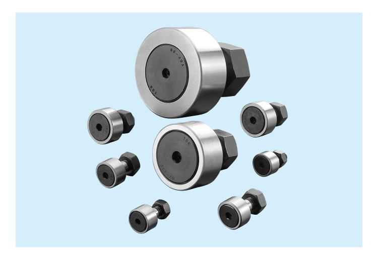
Structure & Advantages The cam follower is a compact and mighty bearing composed of both the set-in needle bearing and a stud. An outer ring contacting the surface of a counterpart rotates smoothly and can do high-speed rotation, too.
