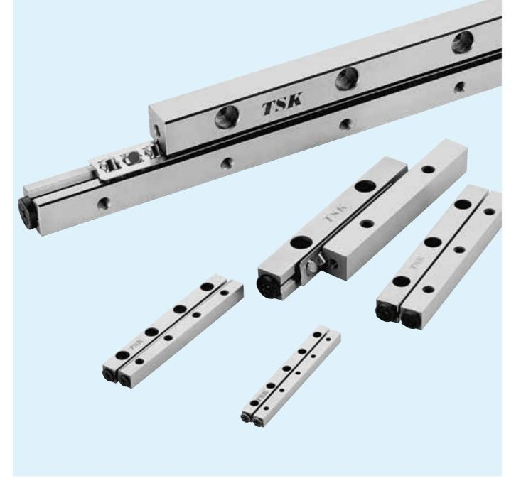
In TSK cross roller silde TCR series, super precision rollers are alternately arranged in between precisely ground V-shaped raceway and tracking base. This enables it to receive loads in any direction and to have high rigidity, very precise, smooth linear motion. This is the most suited linear motion product where high accurate linear motion is required.
